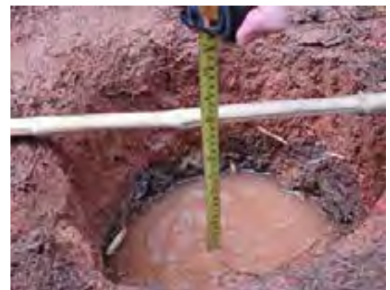
Image 3: Soil Drainage Rate- Percolation test
