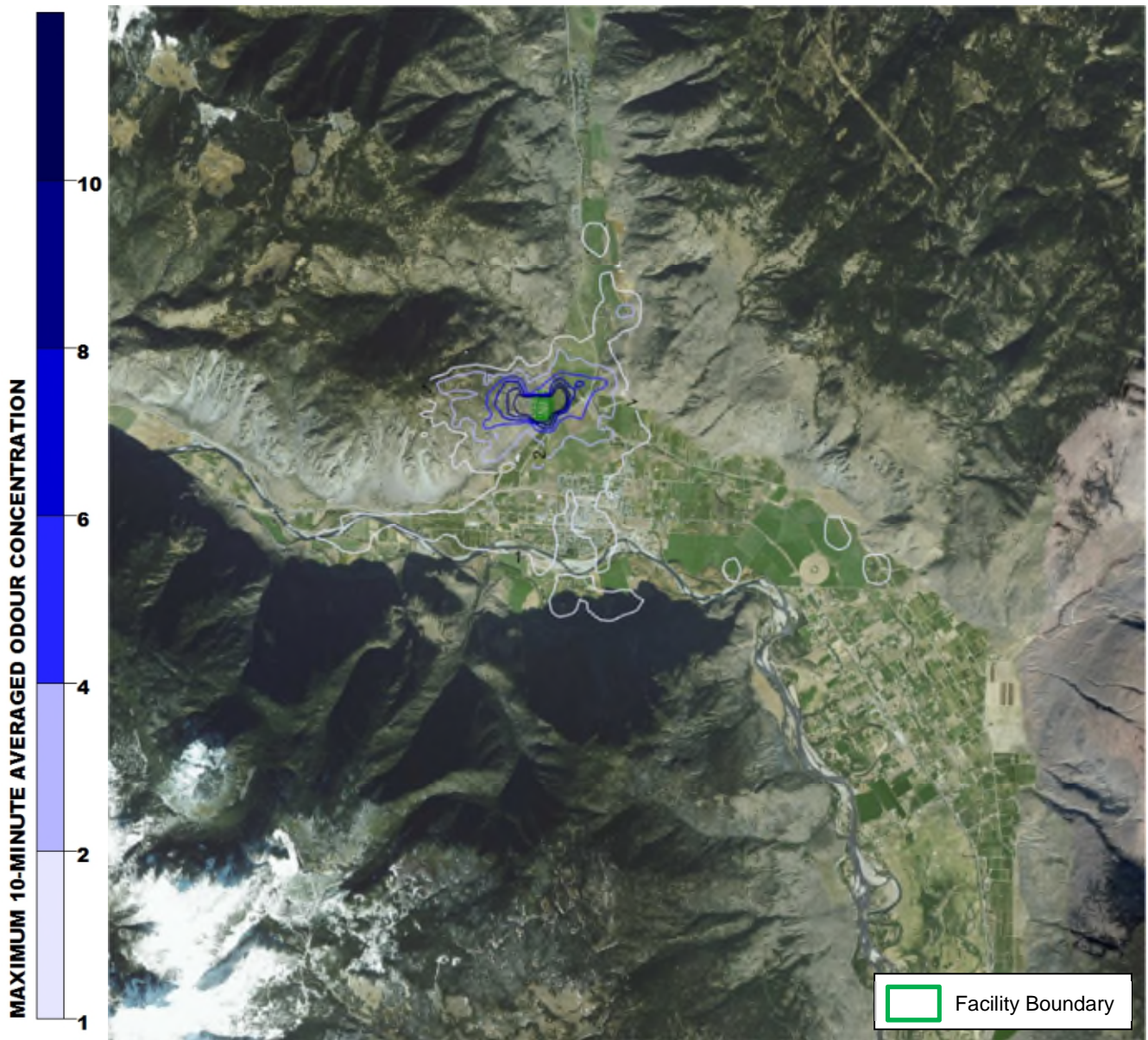
Figure 1: Maximum Predicted Ground Level Odour Concentration (Over a Sustained 10 Minute Period) within the Course of 1 Year (ASP)
