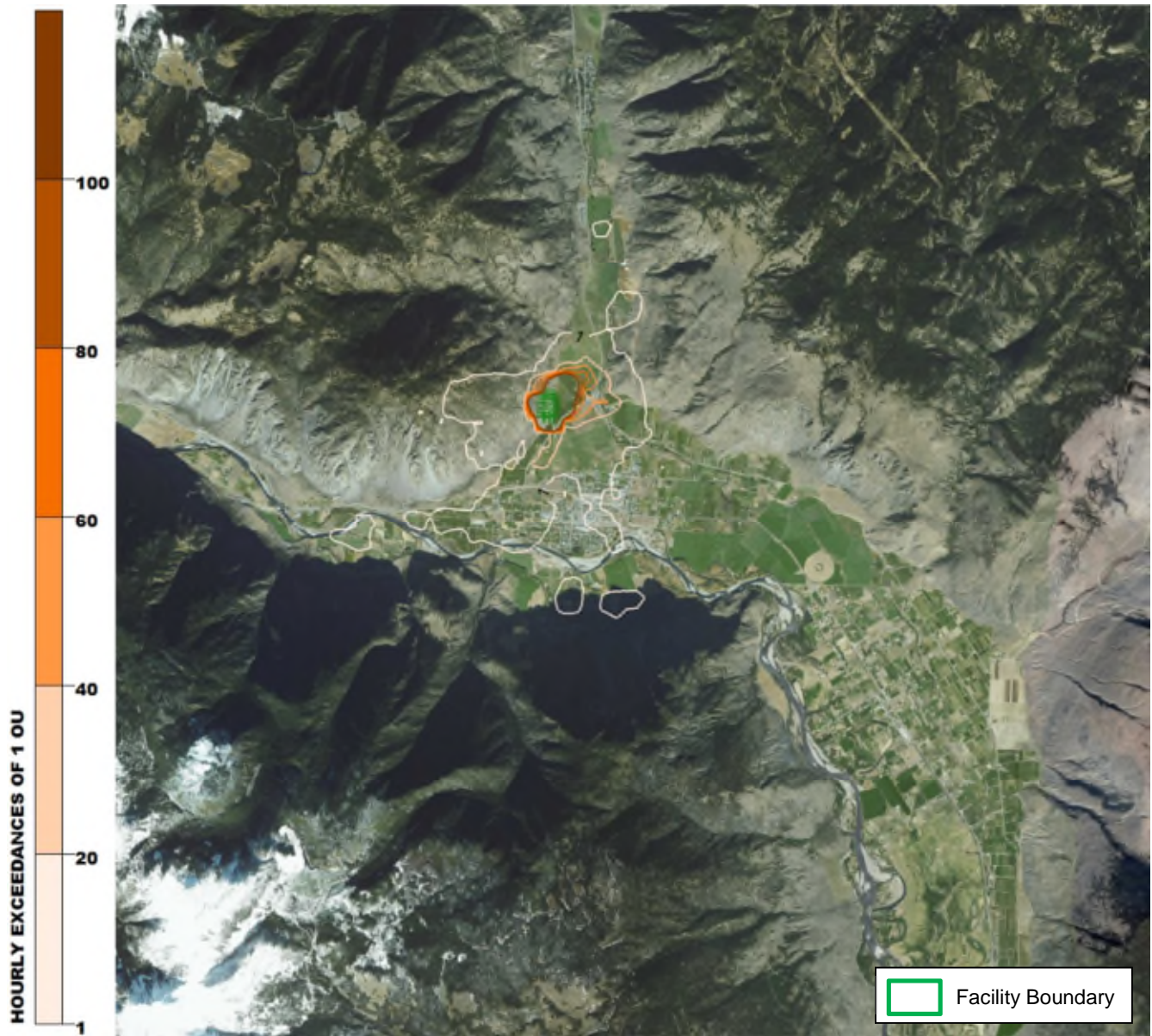
Figure 2: Number of Hours with Exceedances of 1 OU (Detectable Odour by 50% of the Population) within the Course of 1 Year (ASP)
