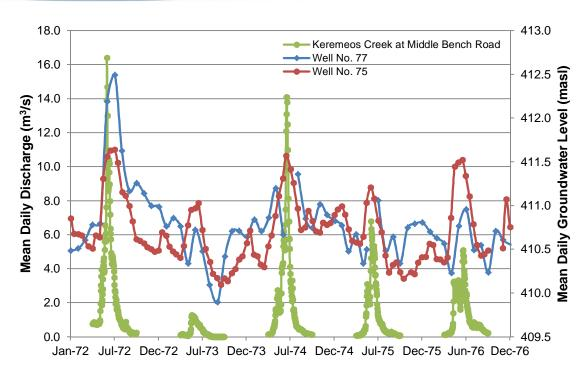
Figure 2-3 Streamflow and groundwater level comparison for Sub-basin #7 (Keremeos Creek), 1971-1977
