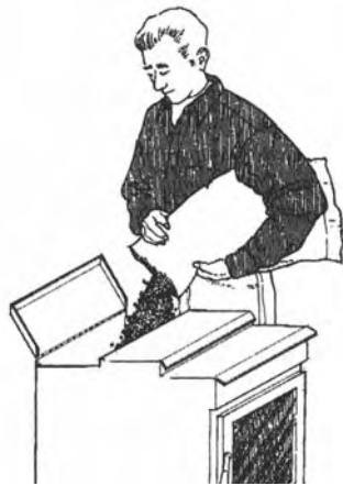
Pellet appliances have some advantages over firewood burning appliances and also some disadvantages. In general, householders looking for convenience, automatic operation and neatness may find a pellet appliance desirable. Those who highly value low cost, self-sufficiency and heating security would find a regular wood stove more suitable.
