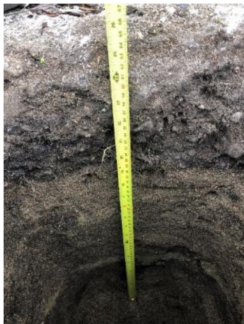
Photo 7 Stratigraphy of SE Wall of ST-4 Showing Soil Disturbance in the Form of Mottled Sediments
