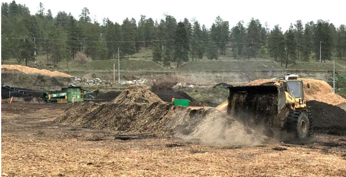
Photo 8 - 'Secondary-mix' for each design mix. A linear stockpile was created to allow for one final blend with the City of Penticton's 'Wildcat' Compost Turner.
