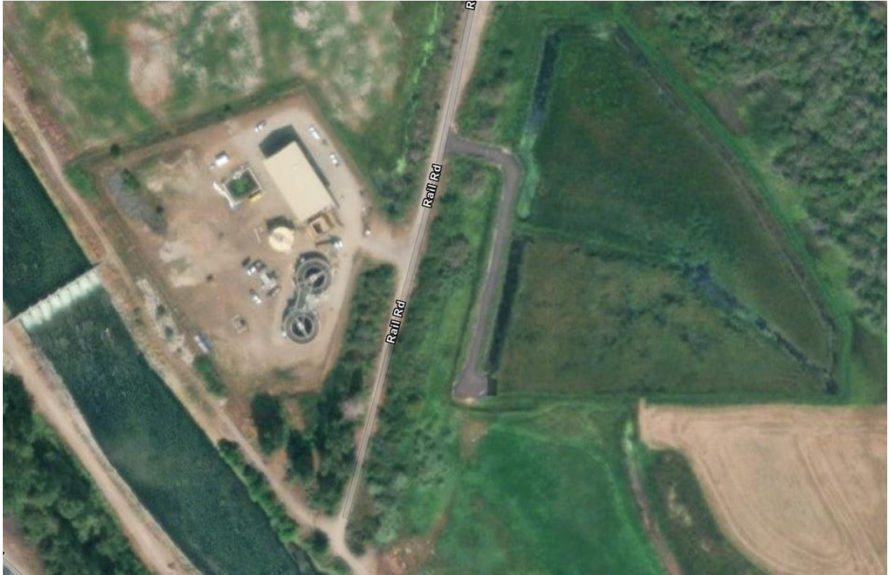
Aerial view of Okanagan Falls Biological Nutrient Removal Wastewater Treatment Facility showing centrifuge dewatering facility under construction in 2022 and polishing wetland located on the right side of Rail Rd.
