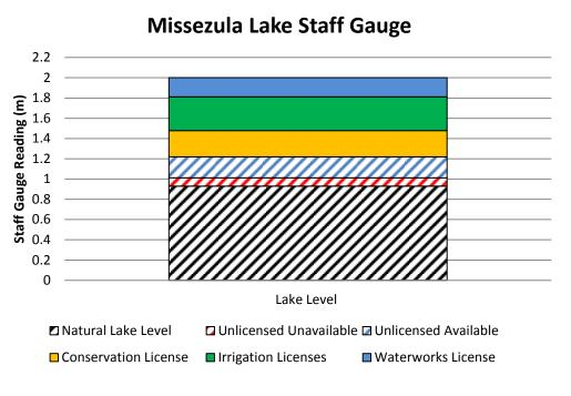
Figure 2. Graphical presentation of the storage volume and associated staff gauge readings
