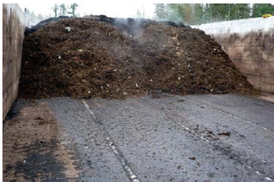
Photo 3.1: Aerated Static Pile
