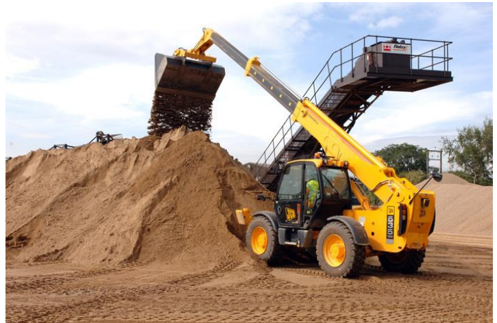
Figure 3.3: Example of a telescopic handler
