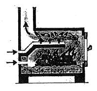
Noncatalytic Stoves - these stoves are designed with baffles and/or secondary combustion chambers which route the burnable gases through the hottest part of the firebox and mix them with sufficient air to burn them more completely.
