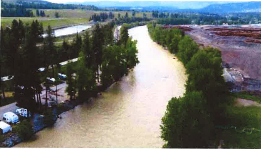
June 1, 2022 – Drone view looking west and upstream along the active floodplain/stream boundary of the Similkameen River adjacent to the property. The stream boundary is noted as the edge of large rooted vegetation.
